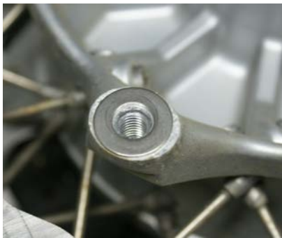
1mm or Large Beveled Washer on stock hub, with BEVELED SIDE UP
